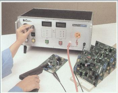
Shown: Component testing using the ARI Model SP02 Safe-T Probe®.
