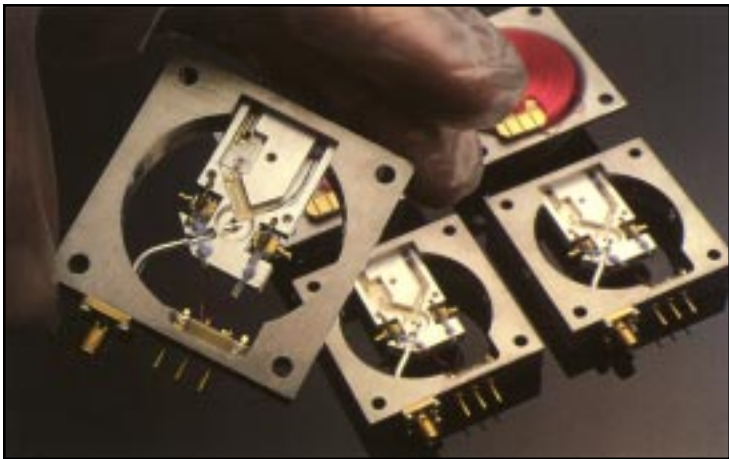
Both the 1230A and 1231A feature Phase Matrix's unique YIG preselected heterodyne down-converter, which provides 10 watts CW burnout protection.
