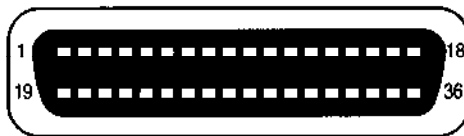
Figure 12b. HP 70611-60010 The standard I/O data cable is a five-foot cable with two female, 36-pin SCSI II type connectors.
